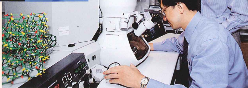
Prof Ning Wang (left) examines 0.4 nm single-walled carbon nanotubes grown in zeolite crystals (see inset) under an electron microscope while Prof Zikang Tang looks on.
